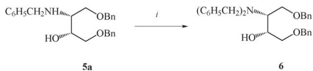
Scheme 3. Reagents and conditions: (i) C 6 H 5 CH 2 Br, Cs 2 CO 3 , toluene/acetone, 90 °C.
